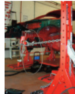
Straight pull on car side with pull tower HD85A
