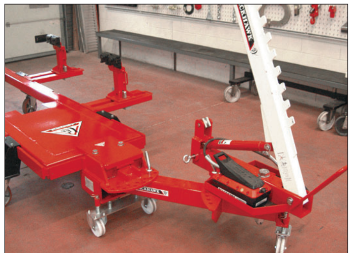
Dozer arm with 2 articulations and 2 sets of holes
